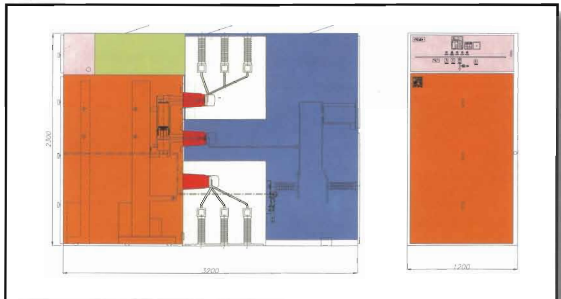
PVP - 702 36kV DOUBLE BUSBAR OUTGOING PANEL
